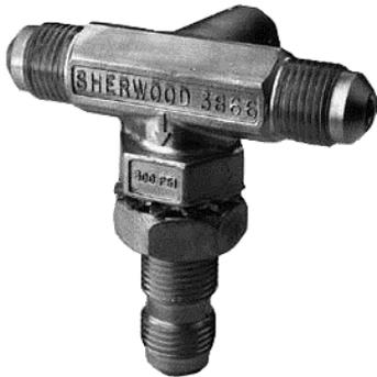
The PV3866 combines a bulkhead with two check valves and a hydrostatic relief valve. This valve is designed to connect two motorfuel tanks to a single line that runs to the fuel lock-off and allows the two tanks to operate at the same time without product flowing from one tank to the other.
