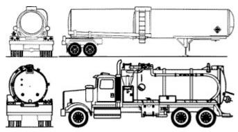
Highway tank for toxic, corrosive and flammable liquids;
