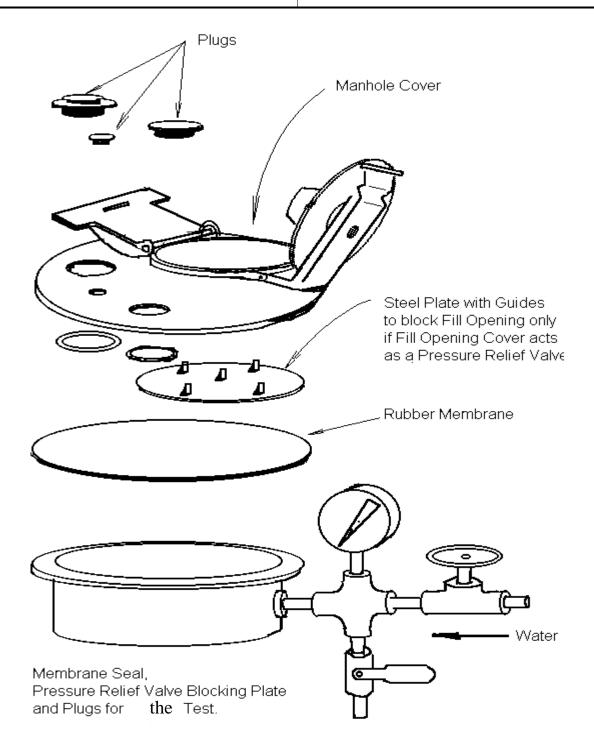
Figure 1 Fixture used in the test.
