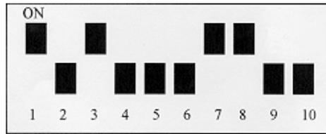
**DIP Switch Settings for the CTM-290 printer.**
