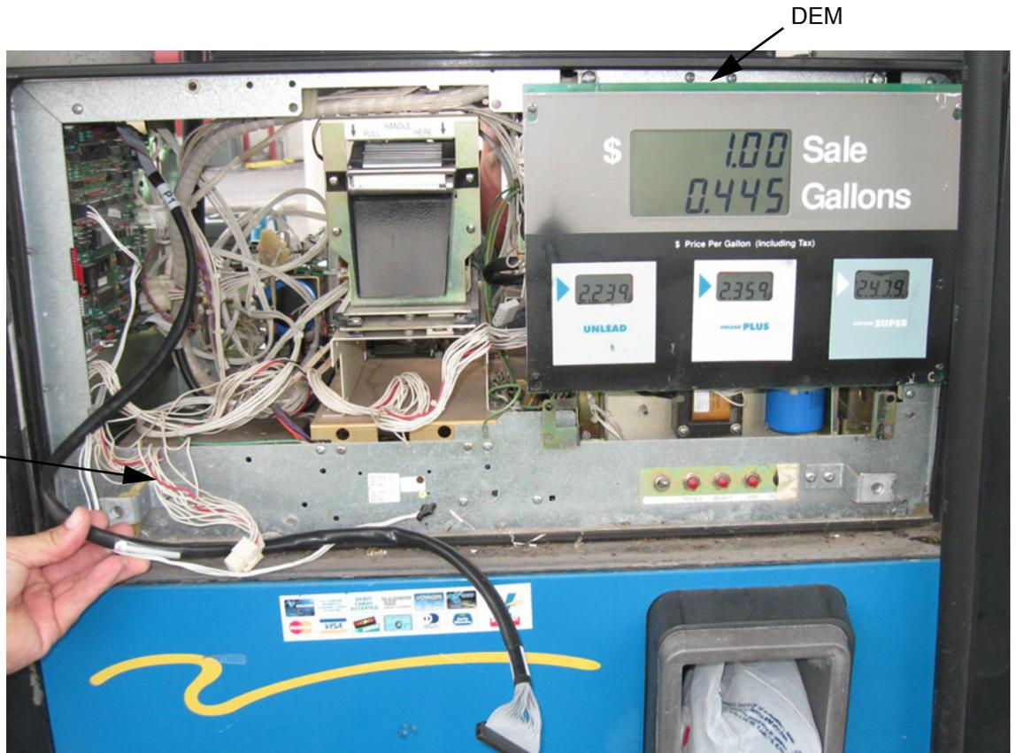
All cables from bezel are removed, including the long PTS cable to the C/c Bd J4 & J5. A new cable is supplied with new bezel.
