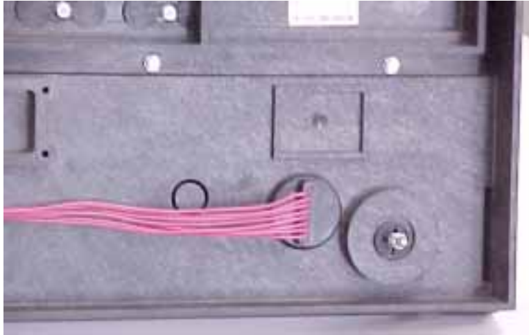
FIGURE 2-11. CASH/CREDIT CABLE CONNECTION TO SWITCH PANEL HARNESS
