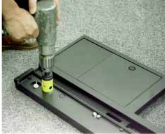
FIGURE 2-7. DRILLING 1-1/2" HOLE FOR THE BEZEL FITTING CONNECTOR (NARROW BEZEL)
