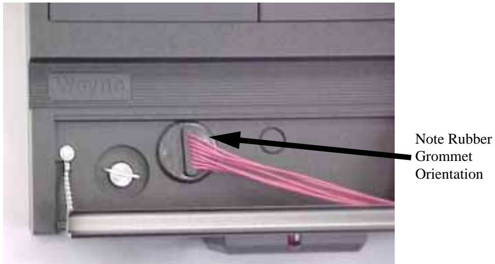
FIGURE 2-10. INSTALLATION OF RUBBER GROMMET (NARROW BEZEL FRONT)
