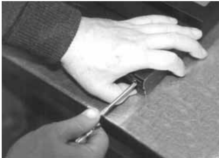
FIGURE 2-4. REMOVING SCREW AND PLASTIC RETAINER THAT SECURE AD PANEL (OPTIONAL)
