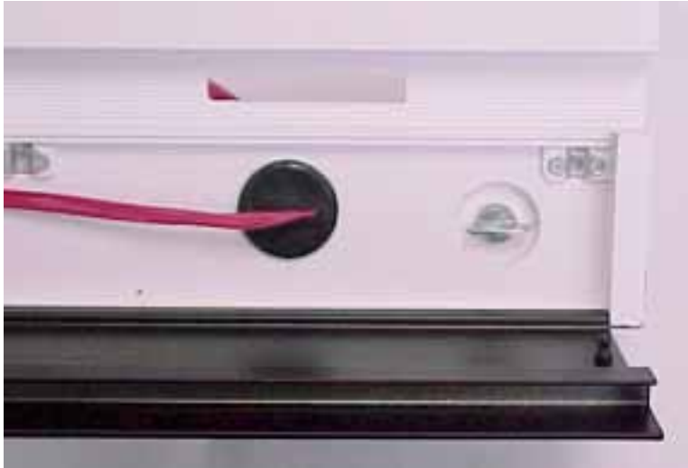
FIGURE 2-9. INSTALLATION OF THE RUBBER GROMMET (WIDE BEZEL FRONT)
