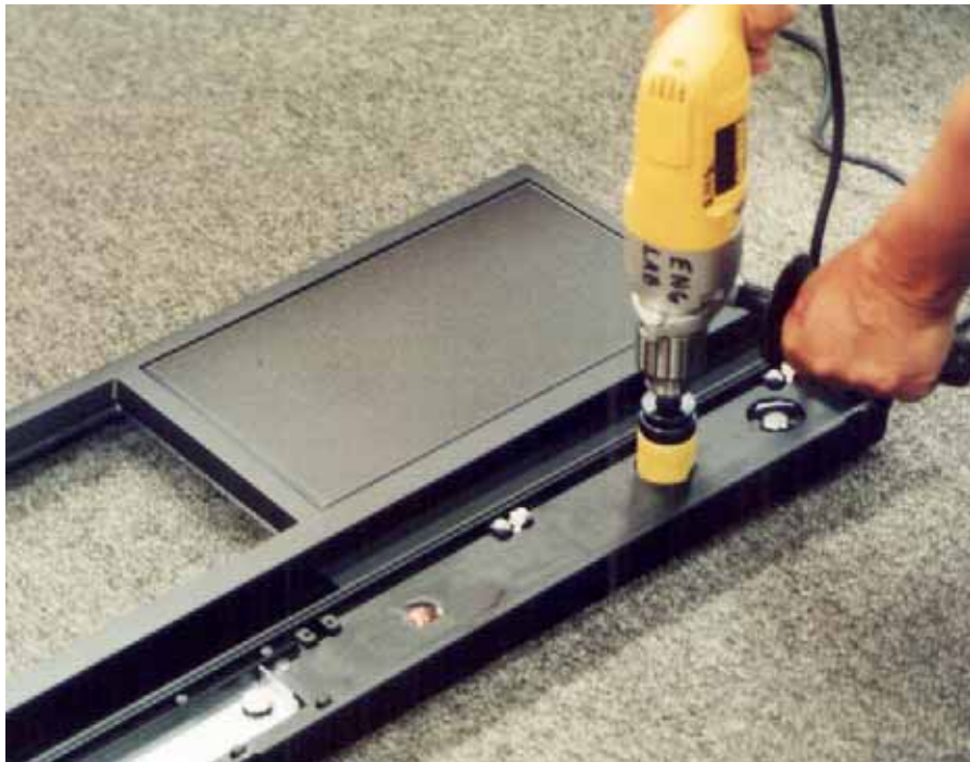
FIGURE 2-6. DRILLING 1-1/2" HOLE FOR BEZEL FITTING CONNECTOR (WIDE BEZEL)
