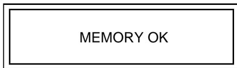
An unsuccessful memory self-test will display one of the following: "BIT 0" through "BIT 7".
