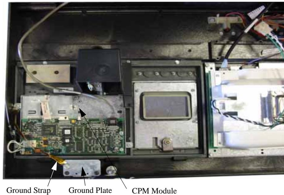
**Figure 2-3 CPM Module Installation**
