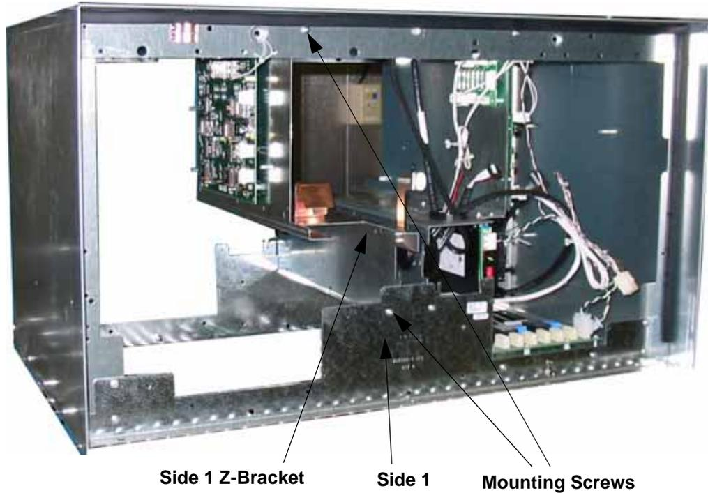
Figure 3-7 Z Bracket with CAT Board Head Mounting Position
