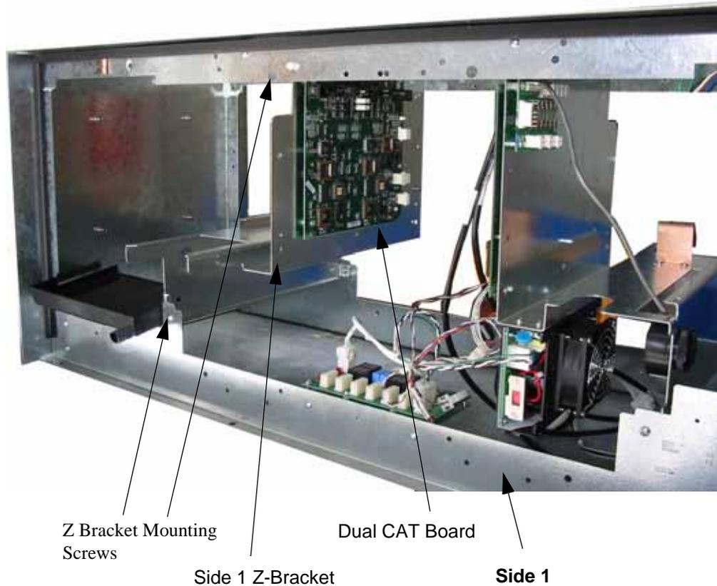
Figure 2-7 CAT Board and Head Mounting Position
