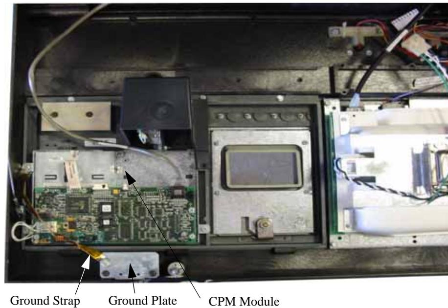
**Figure 3-3 CPM Module Installation**
