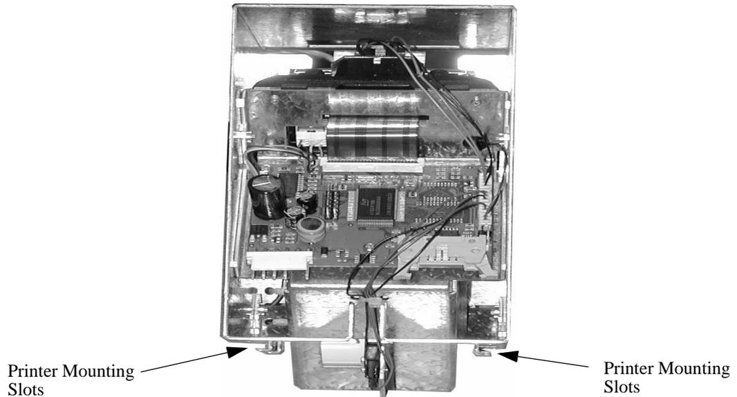
**Figure 3-10 Backside of Clamshell Printer**
