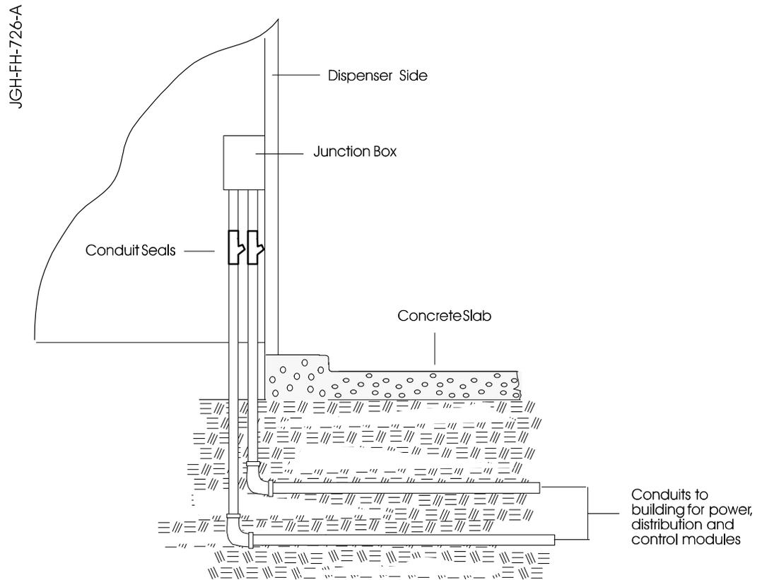
**Figure A- 1 Data and Power Conduit Location**
