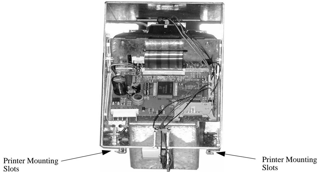
**Figure 2-10 Backside of Clamshell Printer**
