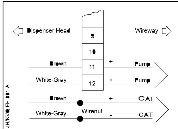
Figure A- 2 Example of Typical Junction Box Connections
