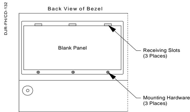
**Figure 3-2 Removing the Blank Panel from the Bezel**
