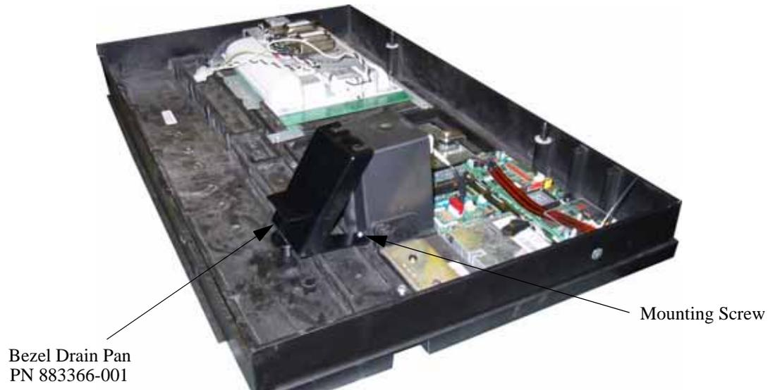
Figure 3-6 Drain Pan Installation
