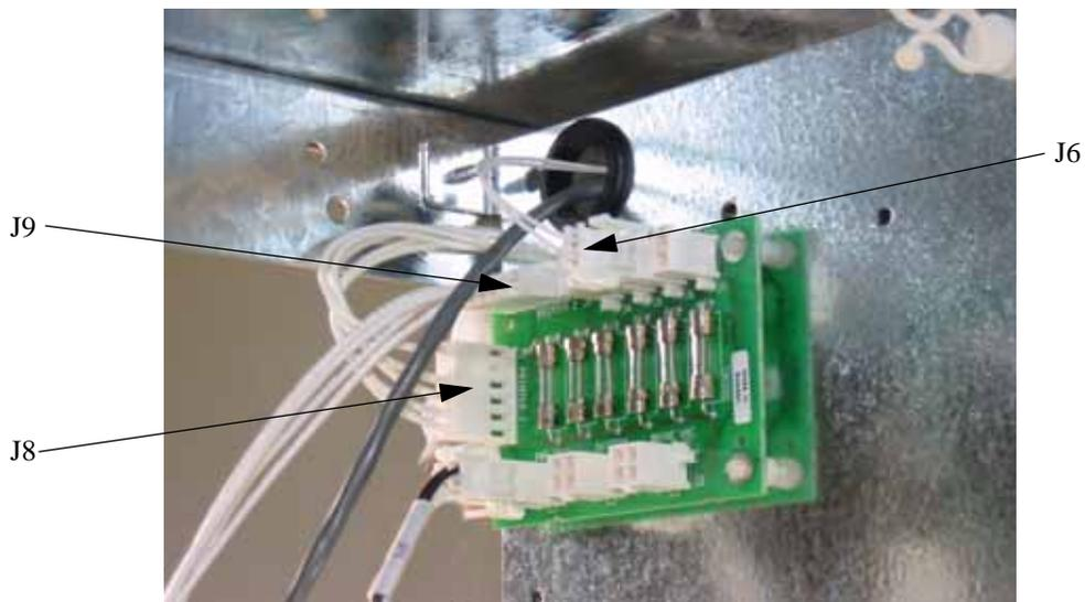
**Figure 2-11 24 Volt Power Distribution Board**
