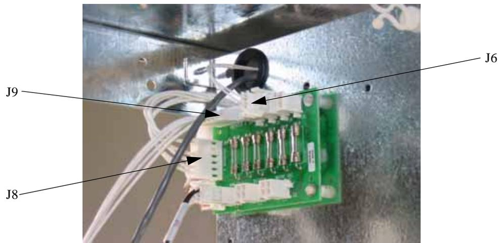
**Figure 3-11 24 Volt Power Distribution Board**
