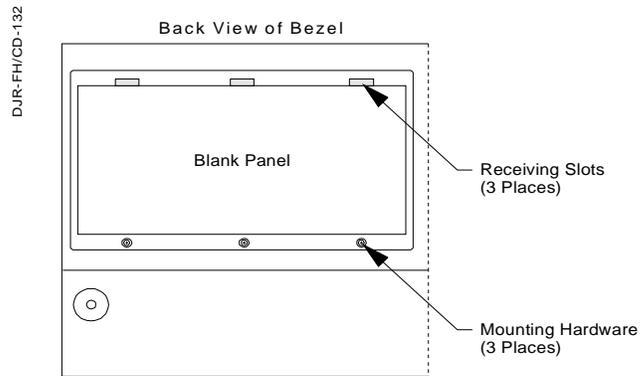
**Figure 2-2 Removing the Blank Panel from the Bezel**
