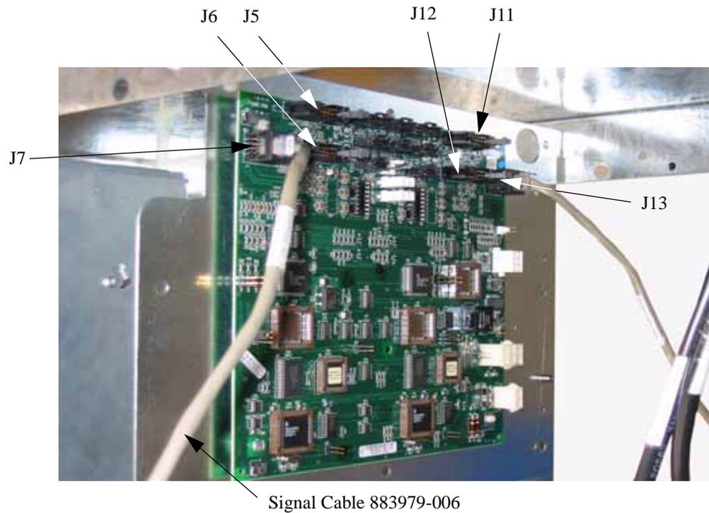
**Figure 2-12 BCB Signal Cable Installation**
