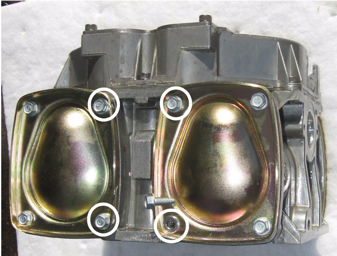
FIGURE 2 INSTALL WASHERS ONLY ON THIS SIDE AND ONLY IN THE FOUR LOCATIONS CIRCLED ABOVE.
