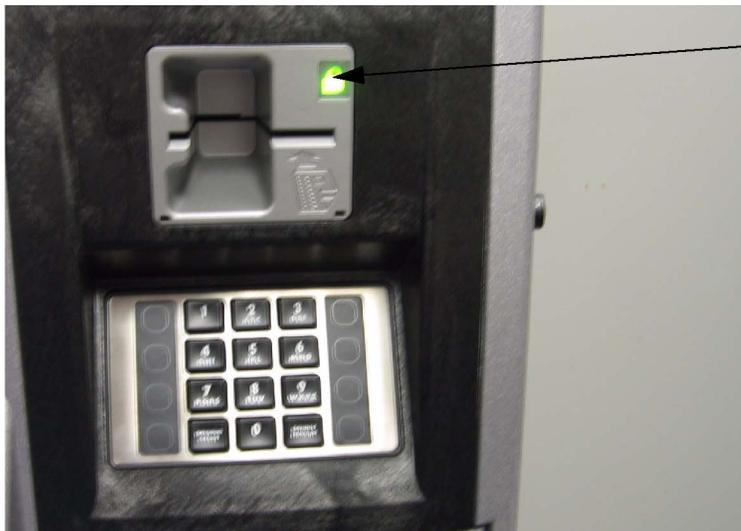
Green Light On ready to accept card during self test. Led goes off when card is removed and track data is received
