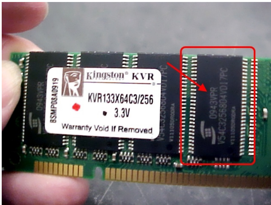
Figure 1: Suspected Defective Memory DIMM, with component chip and letter code VPR highlighted
