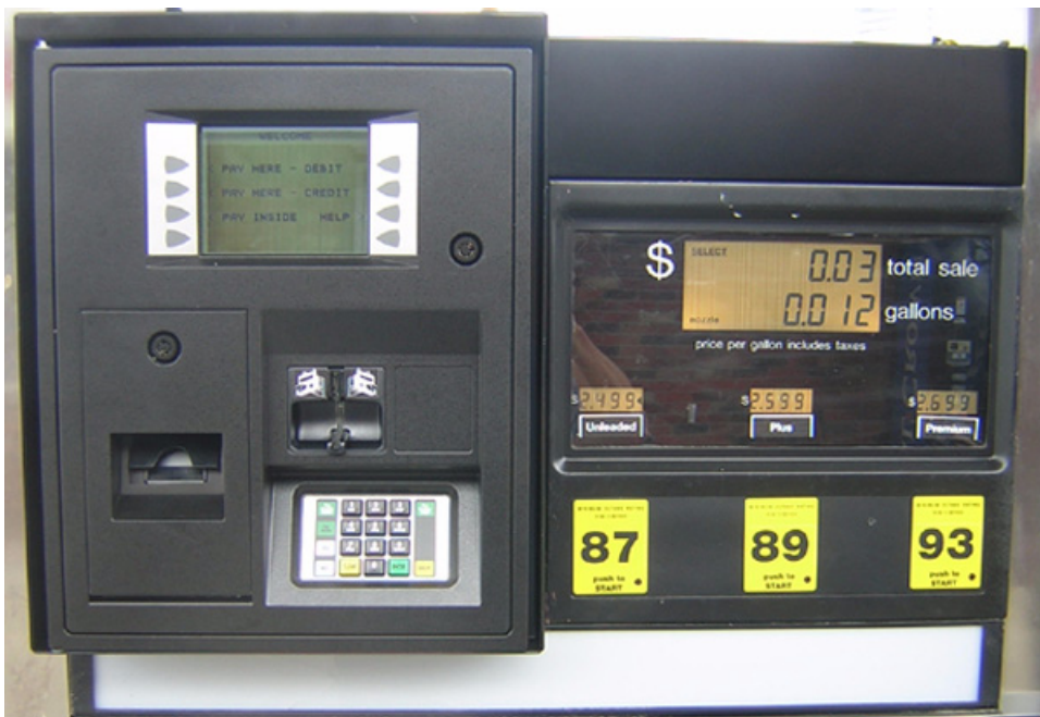
FIGURE 18 Premier B Narrow Body Head After Completed Kit Installation
