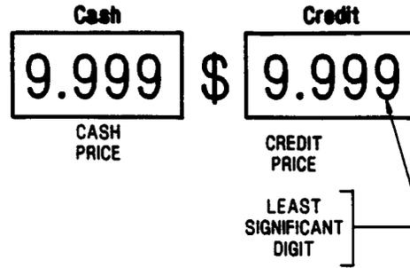
**FIGURE 2-2. UNIT PRICE DISPLAY.** The first closure of the Price Jog push-button causes the least significant digit or tenths of cents position of the unit price to cycle.
