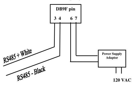
These RS485 wires connect to the 4 Channel CAT GRIB
