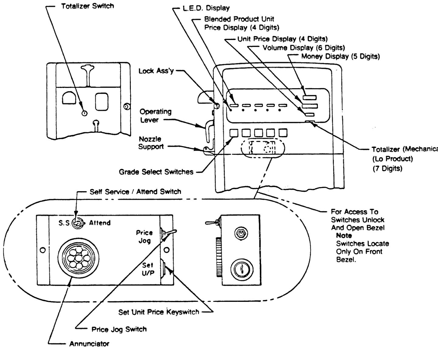
FIGURE 2-4. FUNCTION SWITCH LOCATIONS BLENDING RETROFIT DISPENSERS
