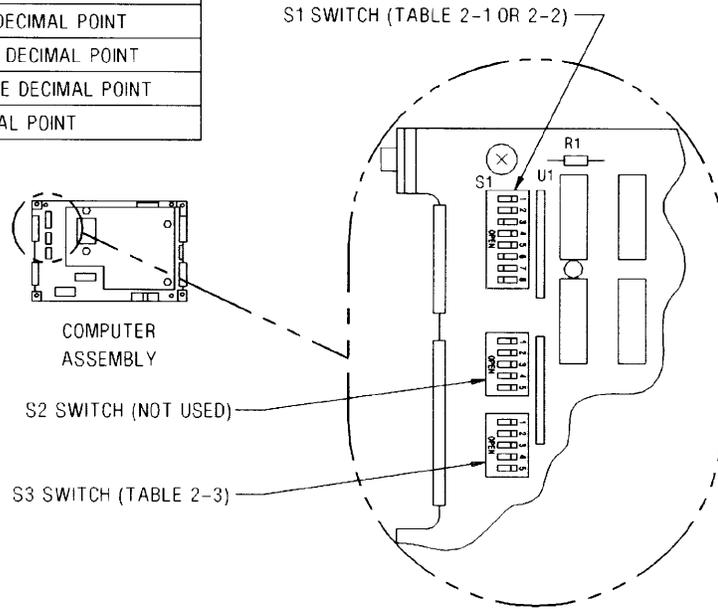
**FIGURE 3-2. SC-82B COMPUTER DIP SWITCH DEFINITIONS**
