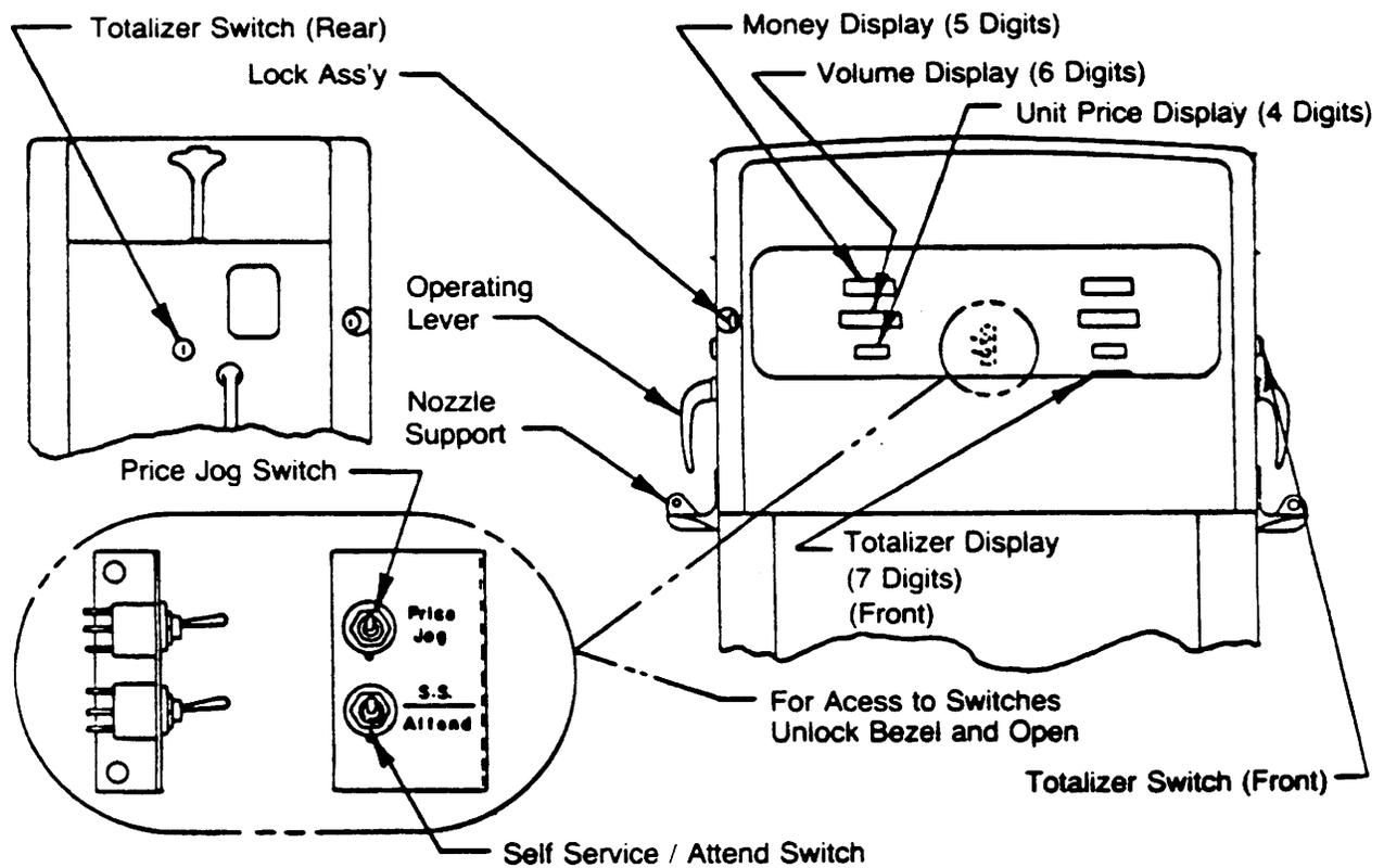
FIGURE 2-5. FUNCTION SWITCH LOCATIONS NON-BLENDING RETROFIT DISPENSERS
