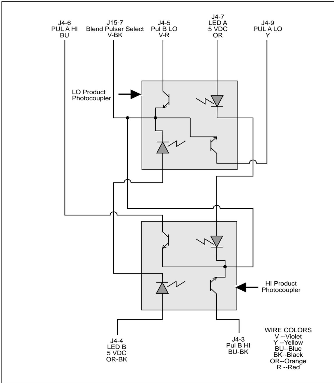
FIGURE 3-3. BLENDING PHOTOCOUPLER WIRING DIAGRAM
