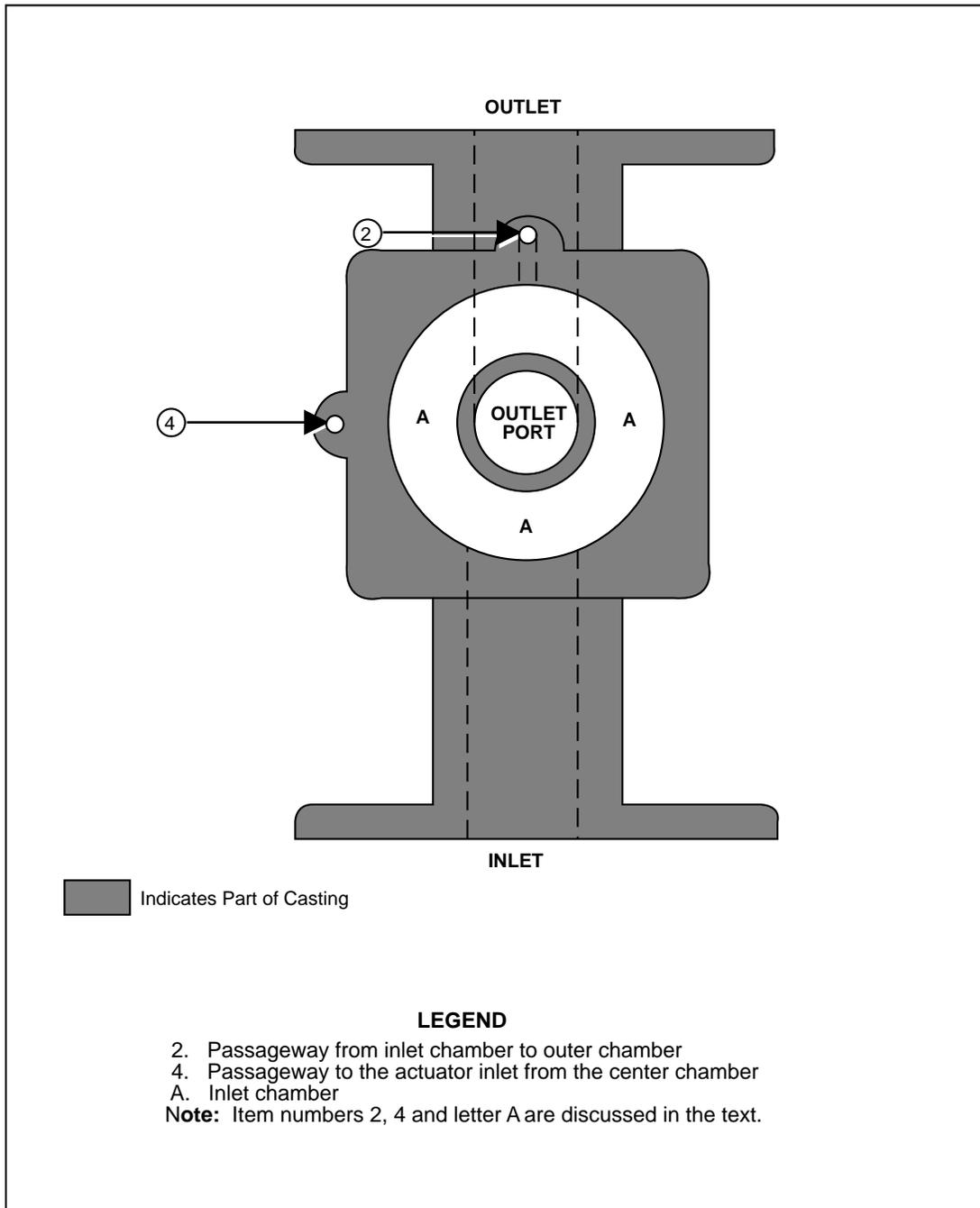
FIGURE 5-2. FLOW CONTROL VALVE WITH KEY NUMBERS 7, 8, 9, AND 10 REMOVED
