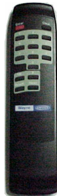
Figure 3-3 IR Remote Control. Use the remote within 12 inches of the display to set unit prices, blend ratios and fueling point ID, read totals, view error codes and other dispenser diagnostic functions.
