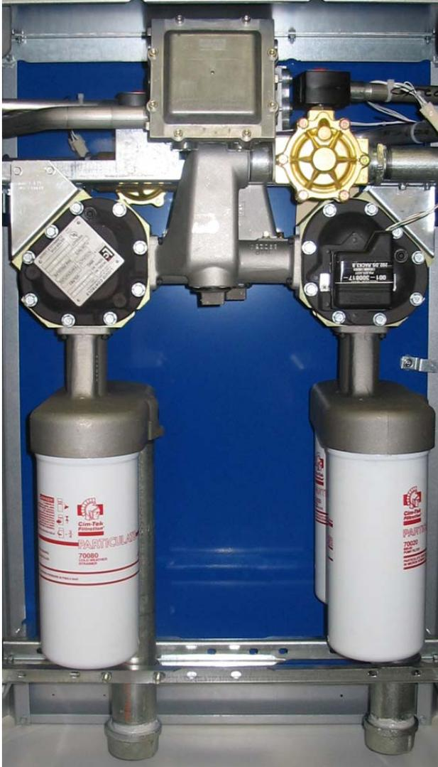
**Figure 1** - View of HS3/V388Dx/4 hydraulics with right inlet reversed for more room when connecting to two satellites.
