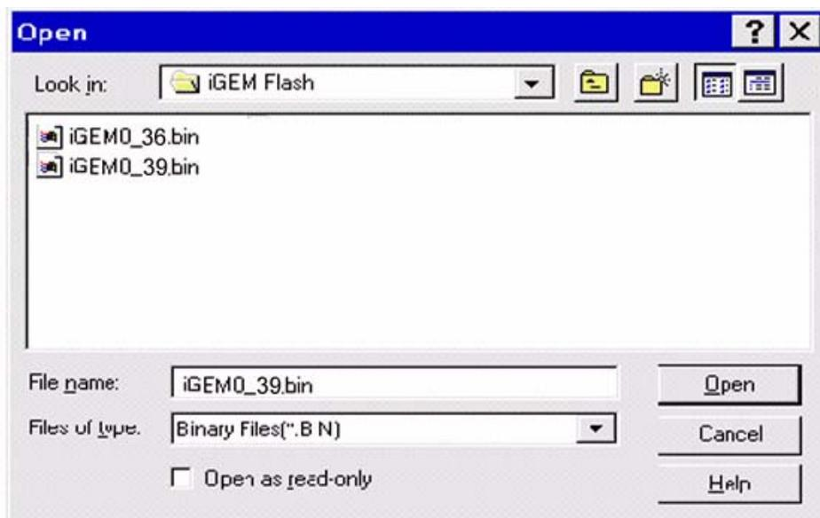
**FIGURE 8-1. SELECTING PUMP CODE FILE.** . Note: When downloading pump code, select the correct pump file name such as, *iGEM\_39.bin*. Do not select flash LDR.bin file as this is not a pump code file.
