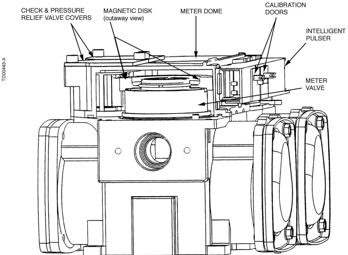
**FIGURE 5-3. iMETER CUTAWAY.** *The magnetic disk affixed to the top of the meter valve is rotated by the meter crank shaft. As the disk rotates, the pulser converts the changing magnetic field into digital pulses.*
