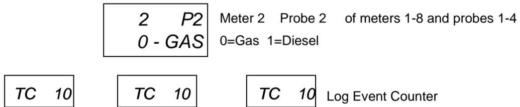
Press the **NEXT** button to view each meter's status for that event or press **CLEAR** and **NEXT** to step through each of the last 10 events.
