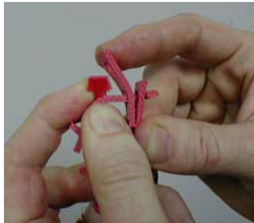
Figure 4-10 Re-Assembling the Link Belt
