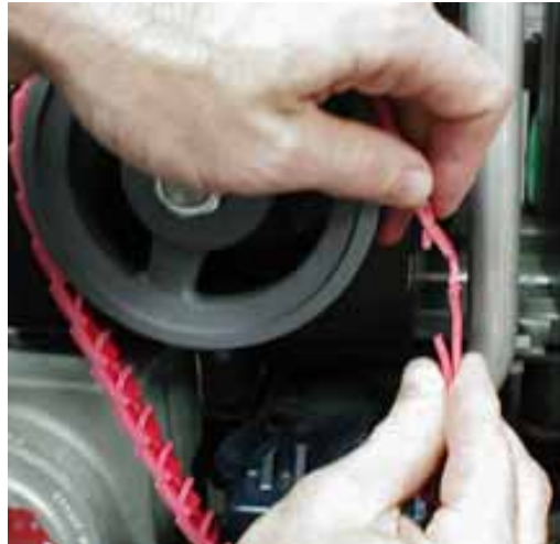
Figure 4-9 Sizing the Link Belt
