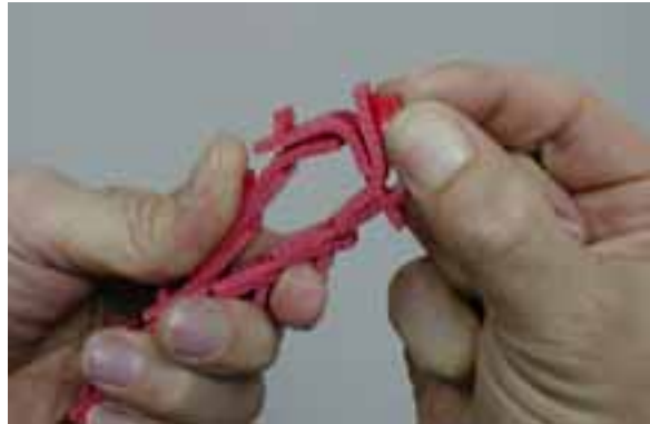
Figure 4-8 Disassembling the Link Belt
