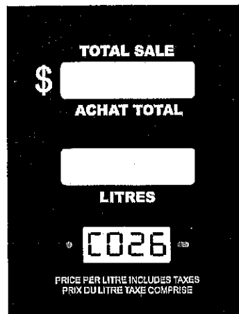
FIGURE 17 - FAULT CODE DISPLAYED BY MICON 500L ELECTRONIC REGISTER
