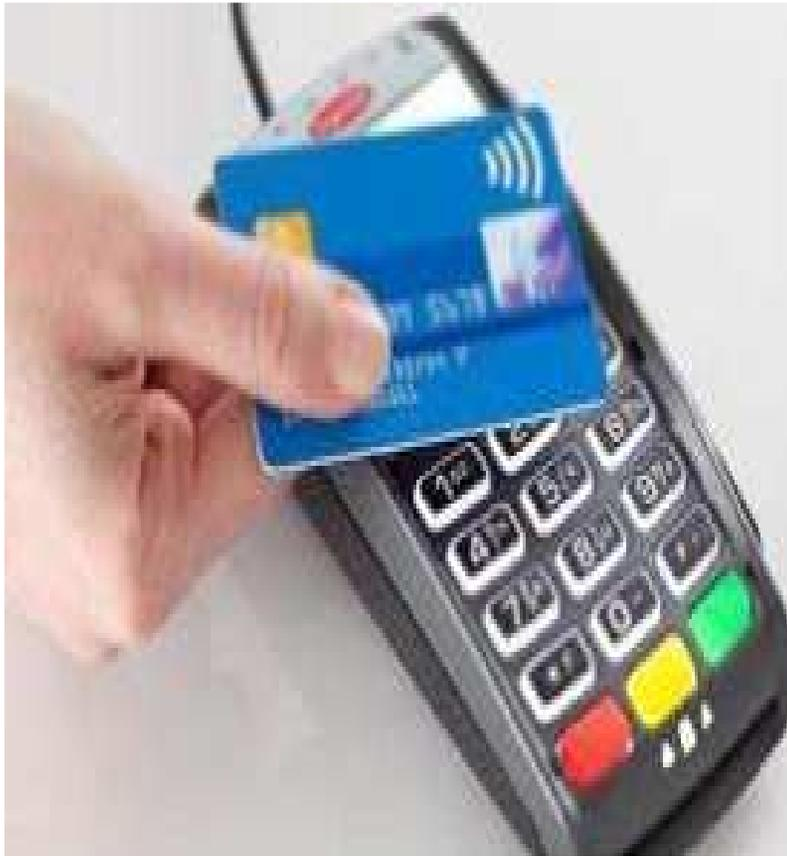
The iPP320 contactless card reader reads contactless payment cards. Hold the contactless payment card close to the active zone around the display. A series of green lights illuminate on the top of the device when the contactless card has been read.
