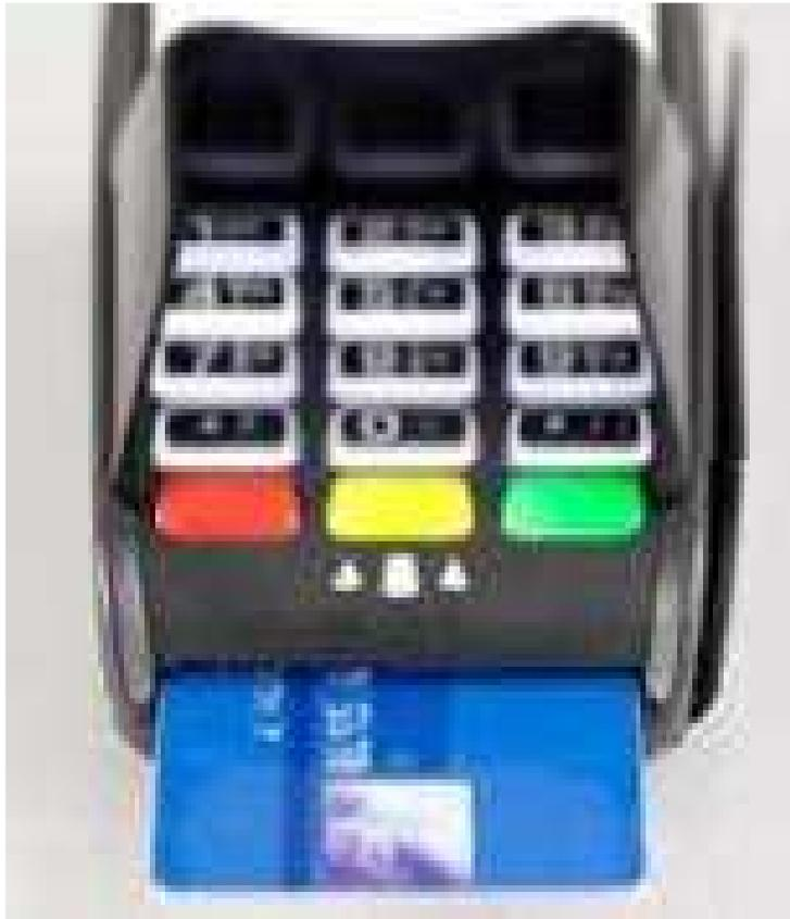
When the application prompts for a smart card, the smart card logos illuminate. Insert the smart card into the slot on the front of the device with the chip facing up and towards the slot. Green lights on top of the smart card reader slot, under software control, can prompt the cardholder when to insert or remove a card. If PIN entry is required, the keypad can also be programmed to illuminate under application control.
