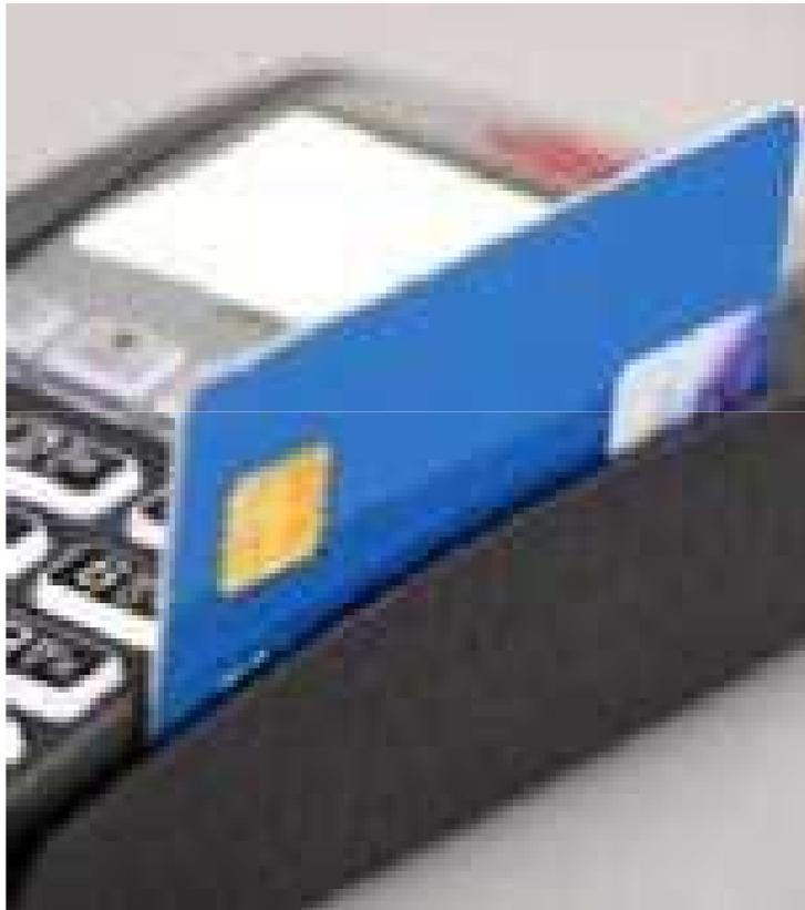
The iPP320 device's magnetic stripe reader reads debit, credit, and all standard magnetic stripe cards. When the application prompts for a magnetic stripe card, the magnetic stripe logo on the top of the device illuminates. Be sure the magnetic stripe side of the card is facing towards the iPP300 graphical display screen. Slide the card in either direction
