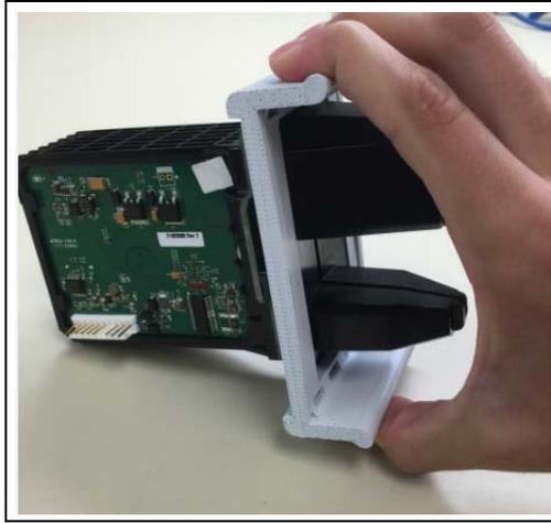
To install the dismount sensor clamp, apply pressure with both the thumb and the fingers to bend the clamp enough to fit the HCR 2 into the clamp as shown in [Figure 9](#). To remove the HCR 2 from the clamp, again apply pressure with both the thumb and fingers to bend the clamp enough to remove the HCR 2.
