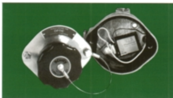
T.I.M. Installed In Scully Overfill Prevention Socket
