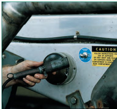
One Connection for Overfill Prevention and Grounding
